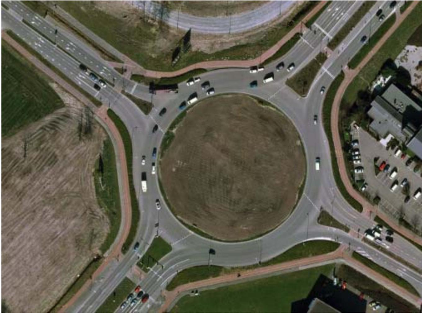
Google shows us the before situation. An enormous traffic lights controlled roundabout with separated cycle paths all around it.
