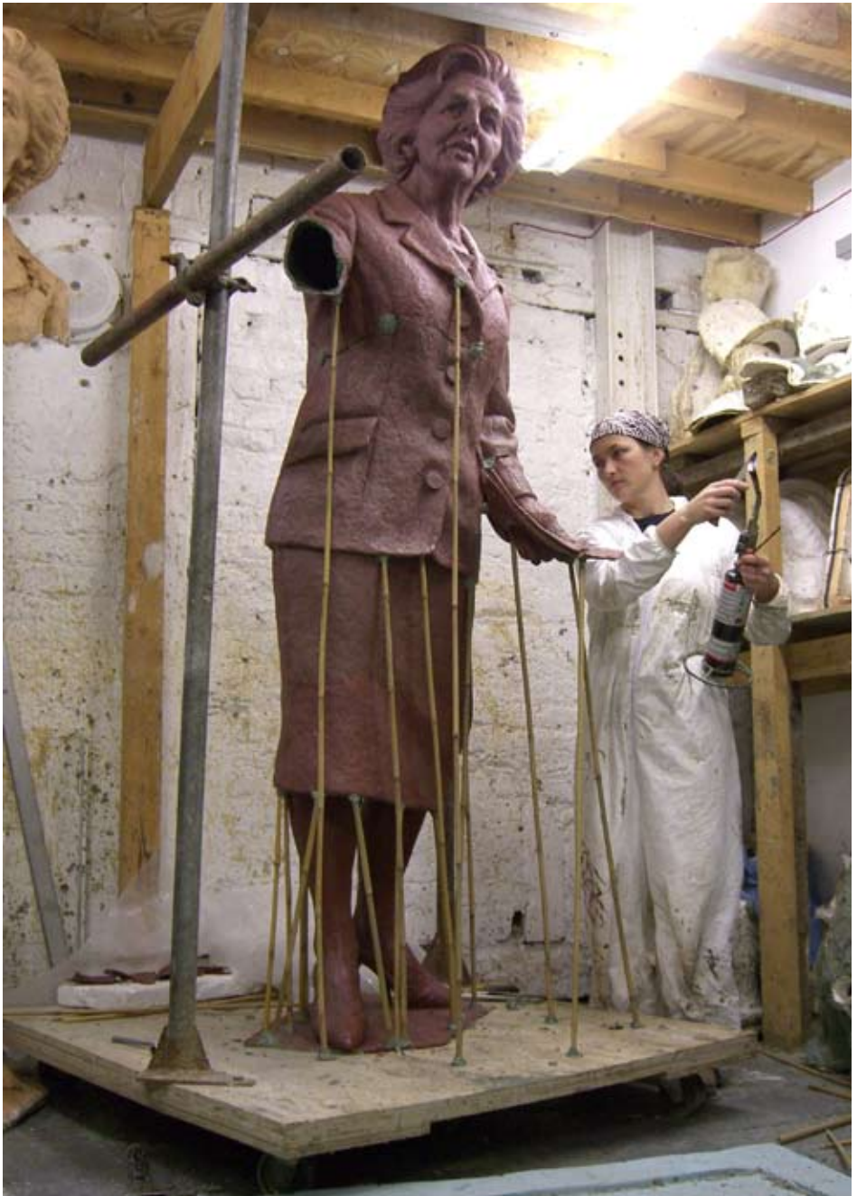
The separate sections of the hollow wax replica are assembled at the foundry to ensure a good fit. Dorota Rapacz prepares to 'weld' the seams, 23 October 2006 (Photo: Antony Dufort)
