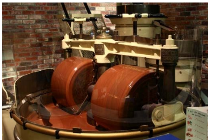
Figure 2 : A chocolate Melanger - Probably one of the oldest nanotools in food processing. Courtesy Sanjay Acharya
